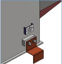
• Earthing connection(s) with a good low resistance is/are essential for adequate protection against electrical faults. All the earth connections should be of sufficient physical size to carry the line current. (Electricity rules and laws to be followed)
