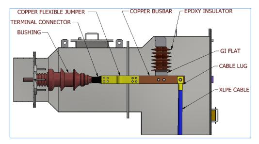
• The cable shall be clamped / supported by suitable cable glands. Care shall be taken to ensure minimal stress on the bus-bar.
