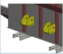
• Skid type under base channels are provided on the bottom of the transformer, having towing holes for pulling & mounting holes for foundation of transformer. For heavy transformers, the under base is equipped with rollers allowing the unit to be moved into final position and then anchored.
