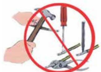
Use a crimp tool. Make sure the stripped cable is inserted all the way into the barrel of the contact and that the contact point is centered in the crimp tool. A crimp tool will effectively compress the contact barrel tightly around the cable strands, allowing them to be pressed tightly against each other and against the inside wall of the contact barrel.
